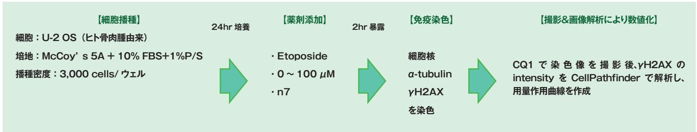
Fig.1 Assay flow of forming  $\gamma$ H2AX with Etoposide within U-2 OS cells nuclei.
